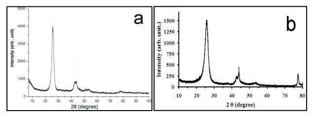
Figure (6): XRD pattern of pure sample of a) SWCNTs, b) MWCNTs.
