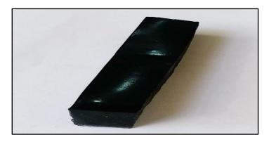
Figure (1): CNTs/epoxy specimen.
