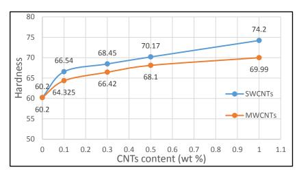
Figure (11): Hardness of CNTs/Epoxy Composites.
