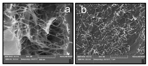
Finally, the images of SWCNTs/epoxy and MWCNTs/epoxy show the alignment of SWCNTs and MWCNTs into epoxy, this means that a good dispersion of each CNTs in this epoxy matrix and this agreement with the results Raman spectroscopy (Qing *et.al.*, 2008).
