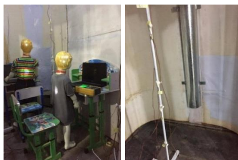
Fig. 14. The layout of the test room for the isothermal (a) The test office room (b) type-II, case-II
