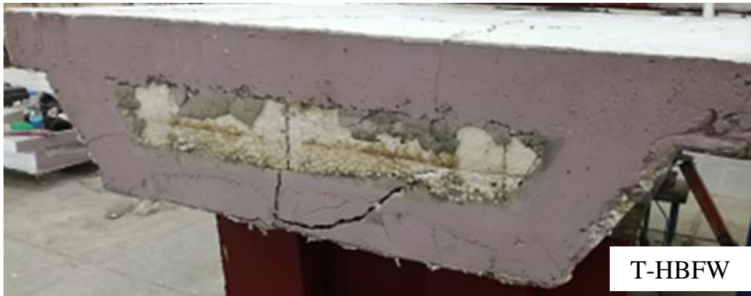
Figure (8): Failure mode of specimen T-HBFW.
