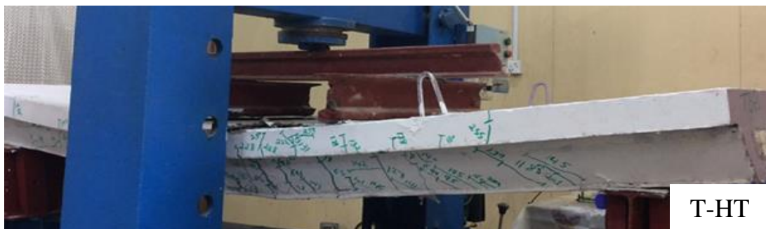
Figure (4): failure mode of T-HT.
