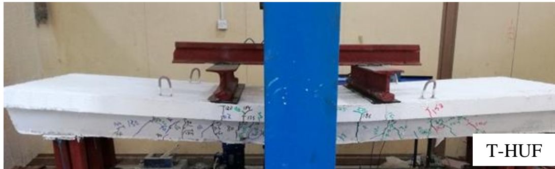
Figure (6): Failure mode of specimen T-HUF.
