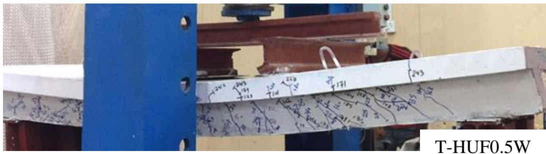
Figure (7): failure mode of specimen T-HUF0.5W.
