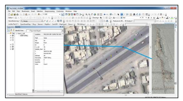
Figure (14) Connect Digital Image to Failure Exist in the Trans. Tining PCC Pavement Surface
