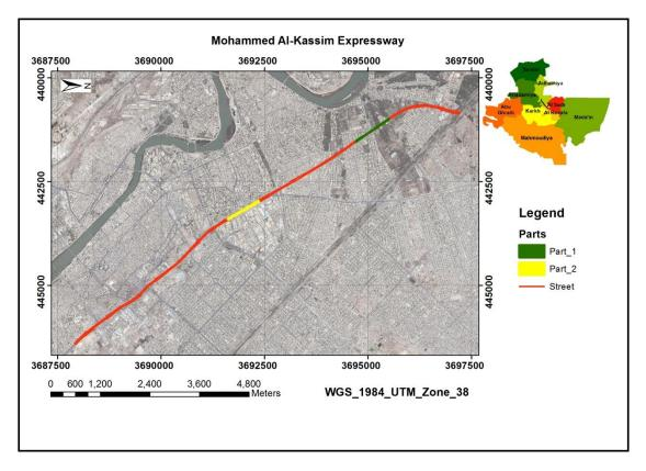
Figure (1) Mohammed Al- Qassim Expressway (Part 1(Transverse Tining PCC pavement surface) Part 2 (AC pavement surface))
