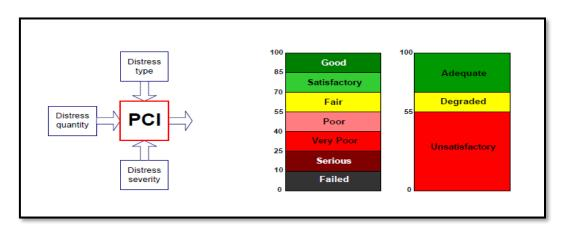
Figure (3) Pavement Condition Index (PCI) requirement, Ranges, and Suggested Colors
