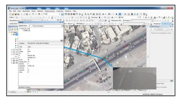
Figure (15) Connect Digital Image to Failure Exist in the AC Pavement Surface
