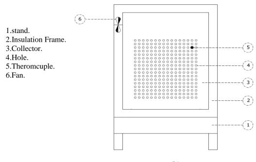
(b) Figure (1): The test rig:
