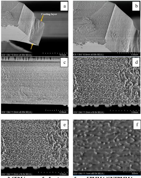
Figure 3 SEM images of a fracture surface of PMMA/CNTPMMA sample Hardness & Elastic Modulus
