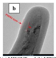
Figure 1 Transmission Electron Microscopy of (a) MWCNT and (b) MWCNT-grafted-PMMA dispersed in THF
