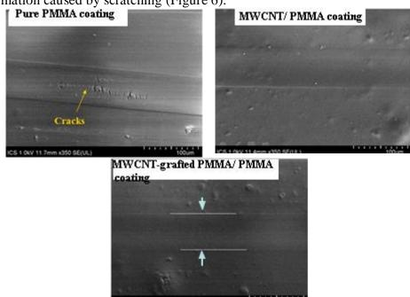
Figure 6 SEM micrographs of the worn surface
