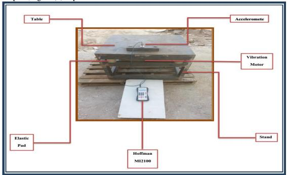
Figure (5) The Vibration Shaker
