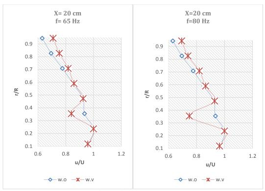
Fig.(2):The velocity profile with different frequency at second position (X=20 cm) for upper
