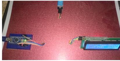
**Figure 5.** An operational system for sensing and reading temperature and humidity levels by using microcontroller
