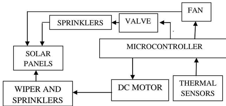
**Figure1.** Block diagram illustrating cooling and cleaning system
