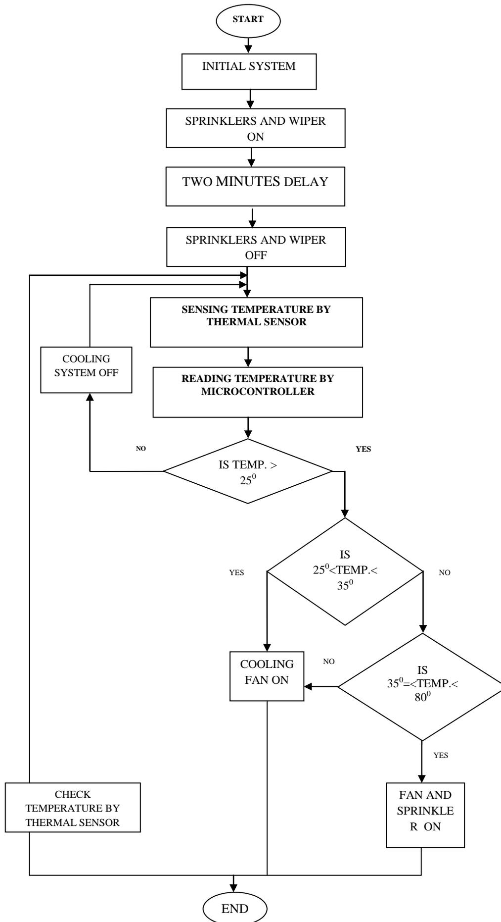
**Figure 4.** Flowchart illustrating the functioning of the cooling and cleaning system.
