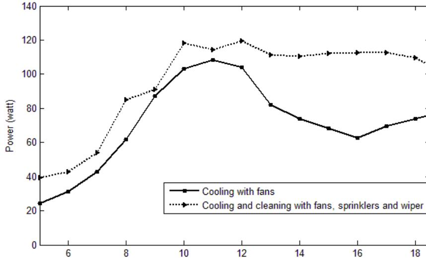
**Figure 7.** Power vs. time for solar panels with fans only compared to solar panels with fans, sprinklers and wipers.
