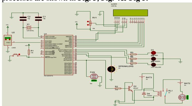
**Figure 3.**Cooling and cleaning system of sprinklers and fans constructed according to proteus program.
