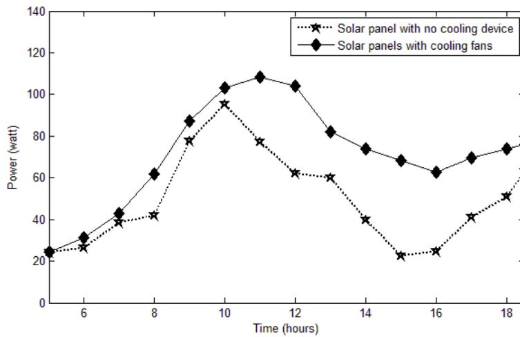
**Figure 6.** Power vs. time for solar panel with no cooling vs. solar panel with cooling fan.
