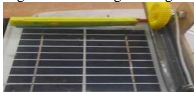
**Figure 2.** Cooling and cleaning system
