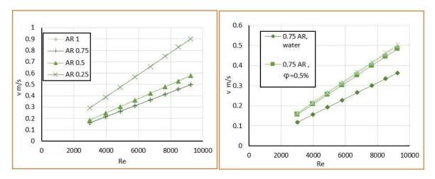
Figure (8): Fluid velocity for different tubes aspect ratio and Reynolds number.
