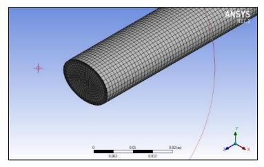
Figure (3): Unstructured used mesh for a 0.75 AR elliptic tube.
