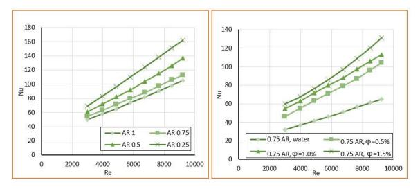
Figure (10): Nusselt number versus Reynolds number at different aspect ratio.
