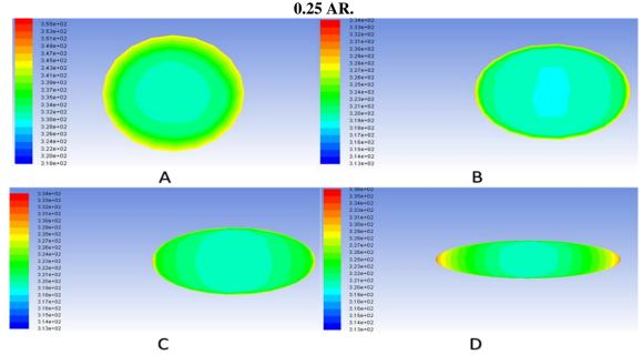
Figure (7): Cross section temperature distribution of elliptical tubes with different aspect ratio at Reynolds number 6743 with uniform heat flux. A) Circular tube, B) 0.75 AR, C) 0.5 AR, D) 0.25 AR
