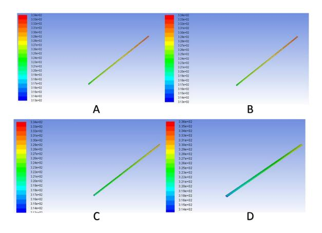
Figure (6): Surface temperature distribution of elliptical tubes with different aspect ratio at Reynolds number 6743 with uniform heat flux: A) Circular tube, B) 0.75 AR, C) 0.5 AR, D)
