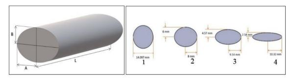
Figure (1): different tubes aspect ratio. Figure (2): Problem geometry and dimensions. Coordinate system for an elliptic duct.
