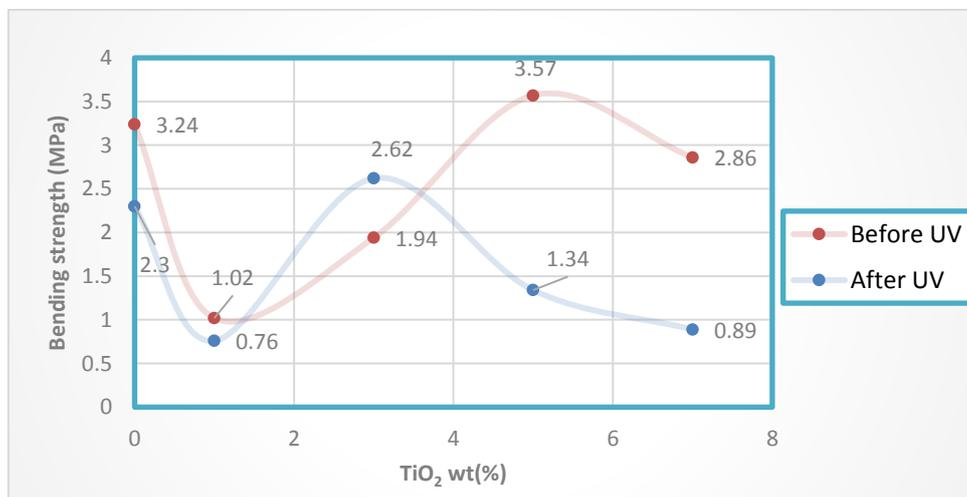
**Fig. (3): Effect of (TiO<sub>2</sub>) nanoparticles and UV radiation on the bending strength.**
