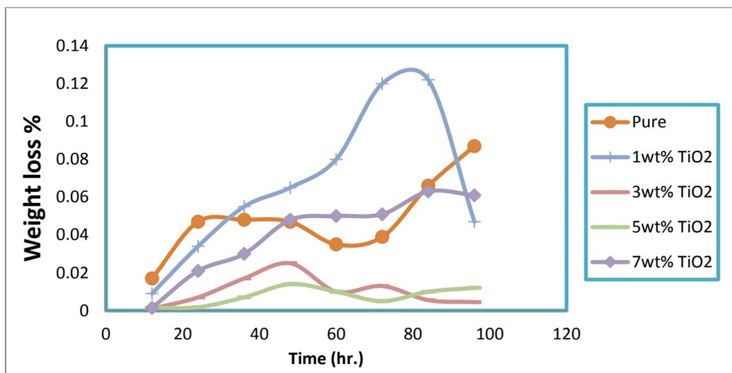
**Fig. (5): Weight loss ratio of all samples with exposure to salt media after UV radiation**
