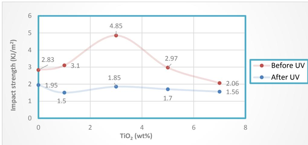
**Fig. (2): Effect of (TiO<sub>2</sub>) nanoparticles and UV radiation on the impact strength**
