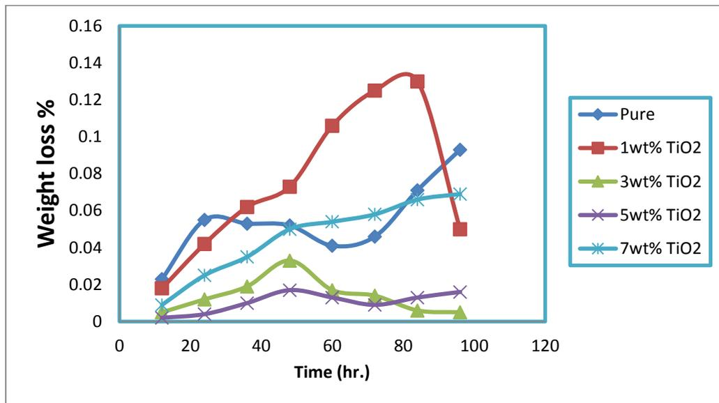
**Fig. (4): Weight loss ratio of all samples with exposure to salt media before UV radiation**
