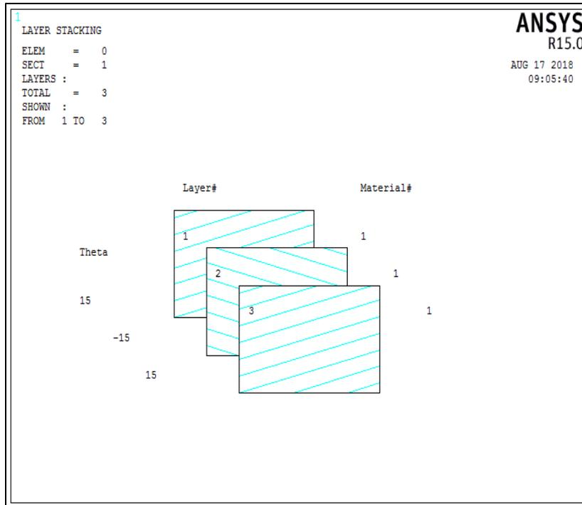
**Fig. 2. Representation of the Lamination angles.**
