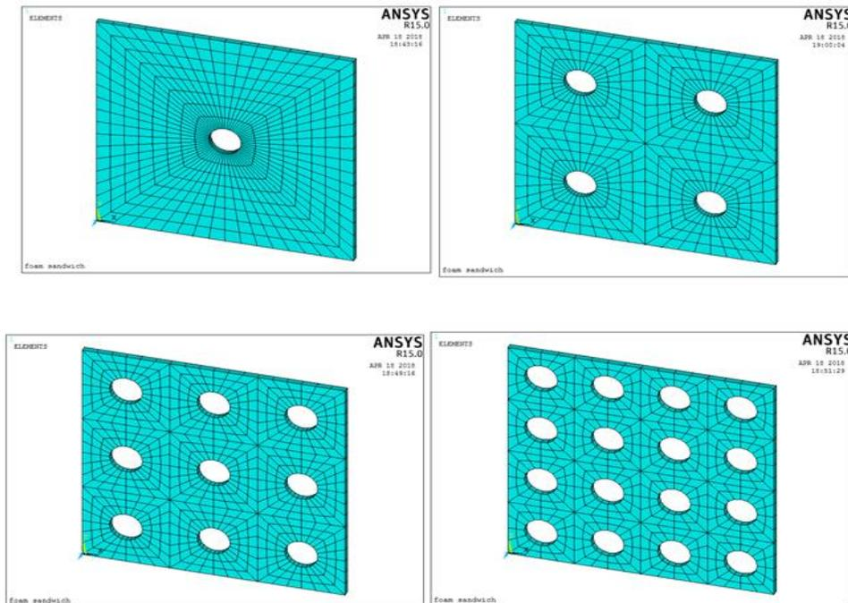
**Fig. (3)Representation of the Meshed Models**
