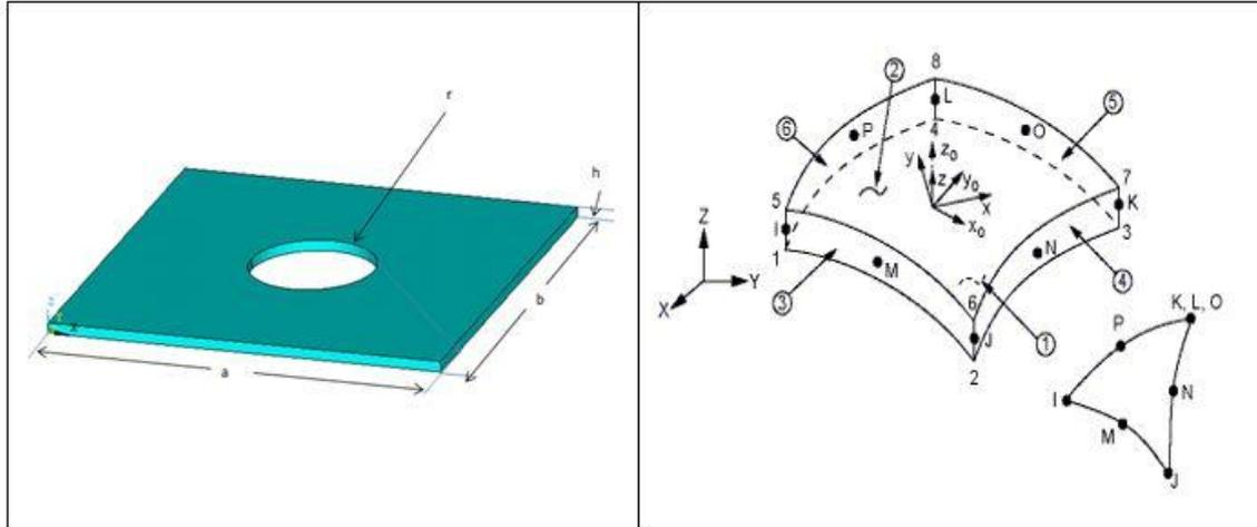
**Fig. (1)Representation of the dimensions model and element type**
