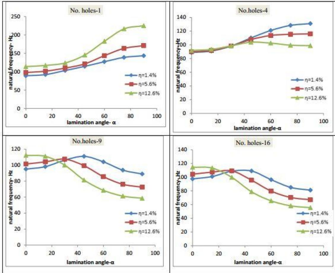
Fig. (6) Variation of frequencies with respect to the lamination angles and holes area ratio for clamped (CCCC) boundary condition.
