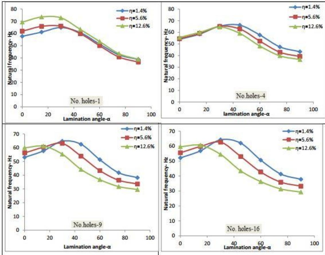
**Fig. (5) Variation of frequencies with respect to the lamination angles and holes area ratio for simply support (SSSS) boundary condition.**
