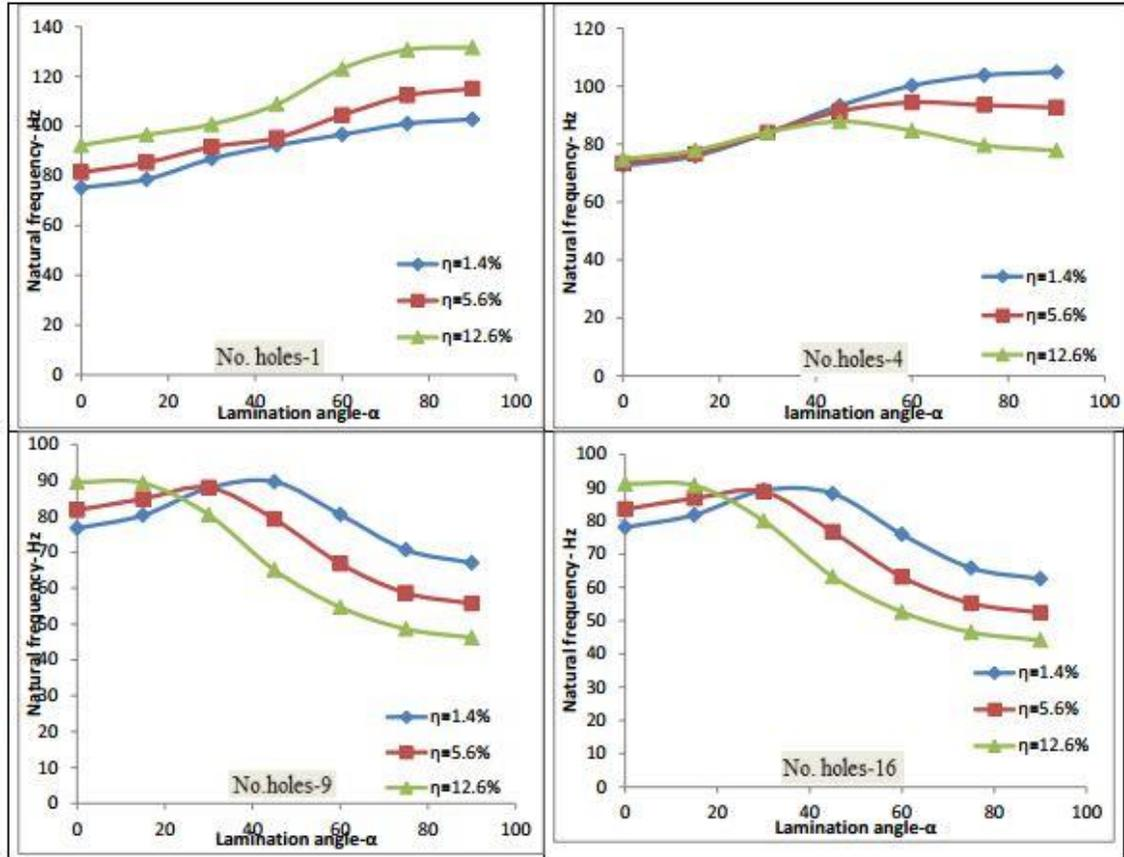
**Fig. (7) Variation of frequencies with respect to the lamination angles and holes area ratio for SCSC boundary condition**
