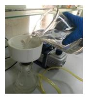
Figure 5 shows the filtration process.
