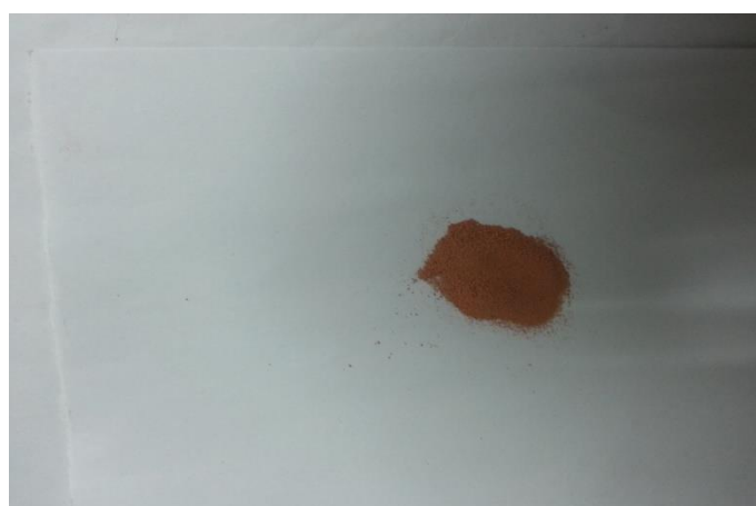
Fig. (3) Deposited copper powder after electrodeposition process
