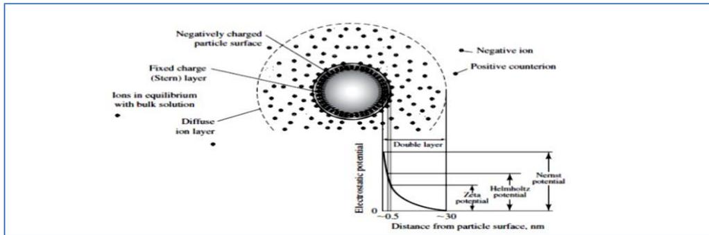
**Figure 2: Electrical double layer (zeta potential) [13]**
