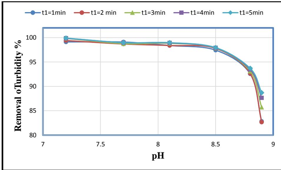
**Figure (6): Effect of pH changes on turbidity removal efficiency with variety of  $t_1$  (set B).**
