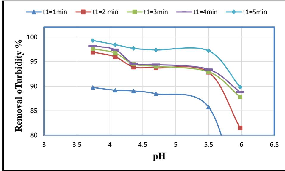
**Figure (4): Effect of pH changes on turbidity removal efficiency with variety of t<sub>1</sub> (set A).**
