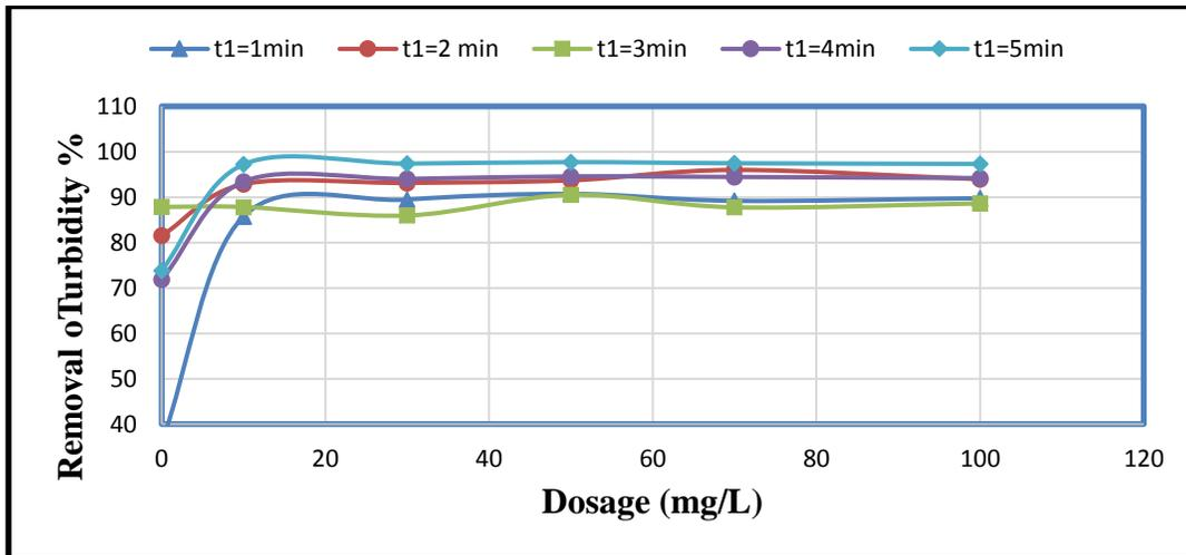
**Figure (3): Effect of alum concentration of turbidity removal efficiency with variety of t<sub>1</sub> (set. A).**
