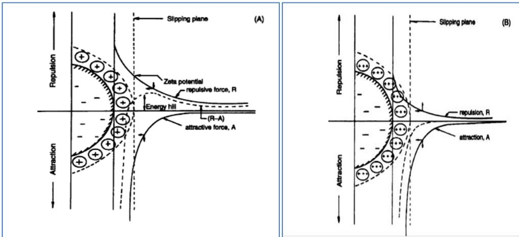
**Figure 1: (A) Particle carries net negative charge and van der Waals positive charge; energy barrier prevents coagulation. (B) Addition of trivalent cations reduces energy barrier, and coagulation is possible. [13]**
