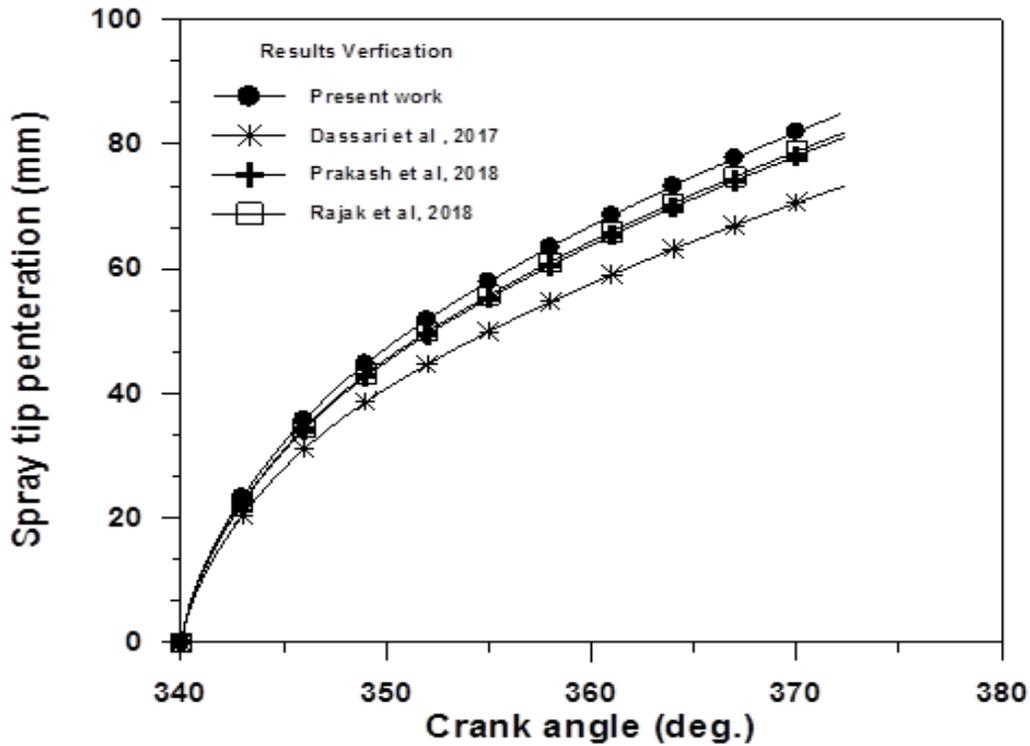
Figure (12) Variation of spray tip penteration with crank angle at full load
