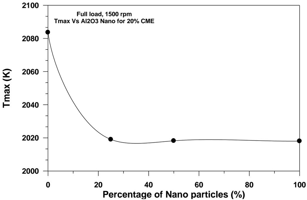
Figure (4) Variation of maximum cylinder temperature with percentage of Nano particles
