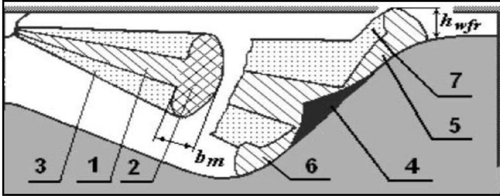
**Fig. (1) Distinguishing areas of the fuel spray[17]**
