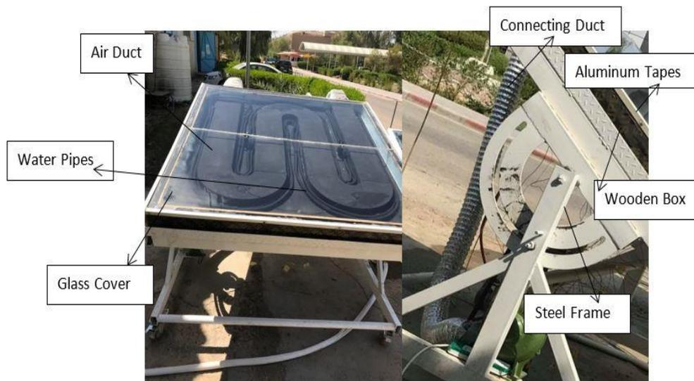
Fig. (1) The Test Rig
