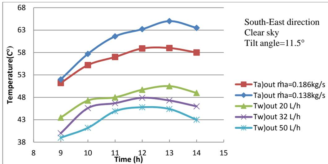
**Fig (7) effect of flow rate on outlet (air & water) temperatures**
