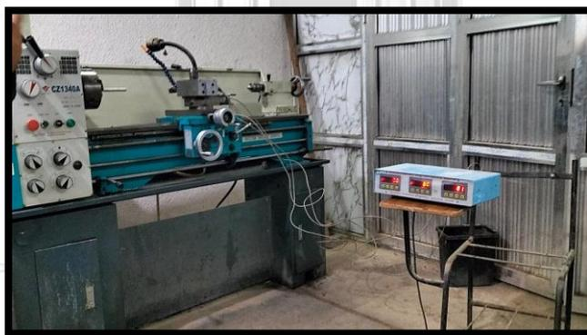
**Figure (7): The Dynamometer and its Amengment on the Lath**
