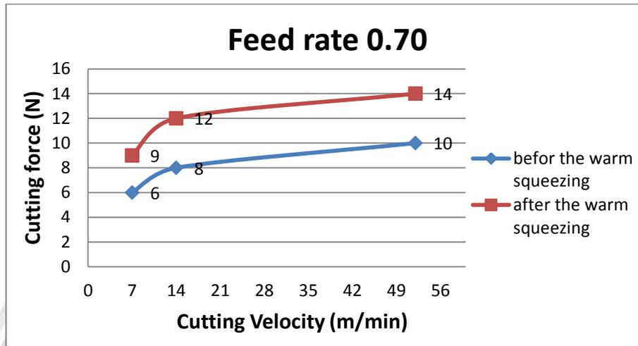
Figures (9): Change of Cutting Force Before and Before Warm Squeezing at a Feed of 0.70 mm/rev
