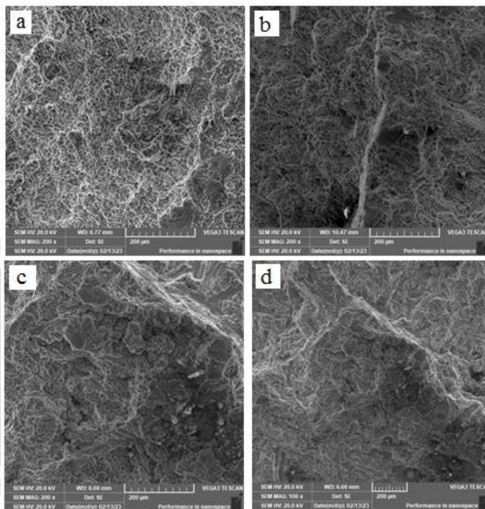
**Figure (6): SEM Images of the Fracture Shape : (a) Heat Treated and Tested at 20°C; (b) Heat Treated, Squeezed by 140MPa and Tested at 20°C; (c) Heat Treated and Tested at 300°C; (d) Heat Treated, Squeezed by 140MPa and Tested at 300°C**
