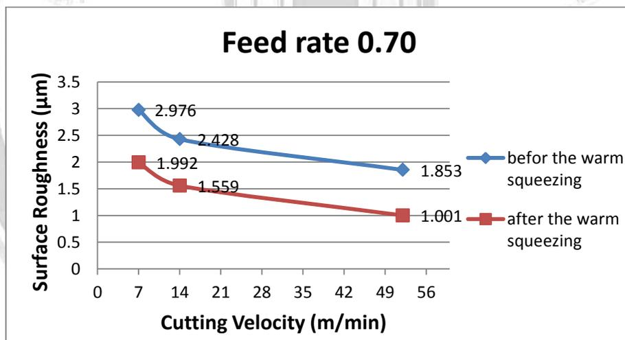
Figures (11): Effect of Cutting Speed on Sample Surface Roughness Before and After the Hot Press Used at a Cutting Depth  $d = 0.2$  mm and a Feed of (0.70 mm/rev)
