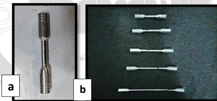
Figure (4): Tensile Specimen (a): Before Testing (b): After Testing Where: Radius of Fillet (R): 6 mm; Gage length (G):  $35 \pm 0.5$  mm; Diameter (D):  $8.75 \pm 0.25$  mm; Length of Reduced Section (A): 45 mm.
