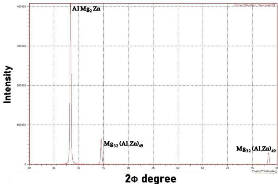
Figure (1): XRD Analysis on the Heat Treated 7075 Al Alloy
