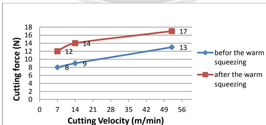
Figures (8): Change of Cutting Force Before and After Warm Squeezing at a Feed of 0.130 mm/rev
