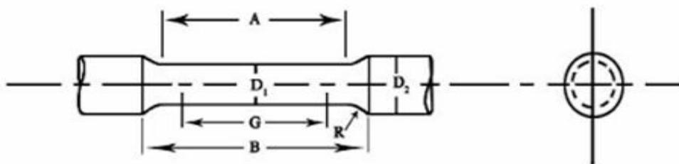
Figure (2): Standard Round Tensile Test Specimen [11]
