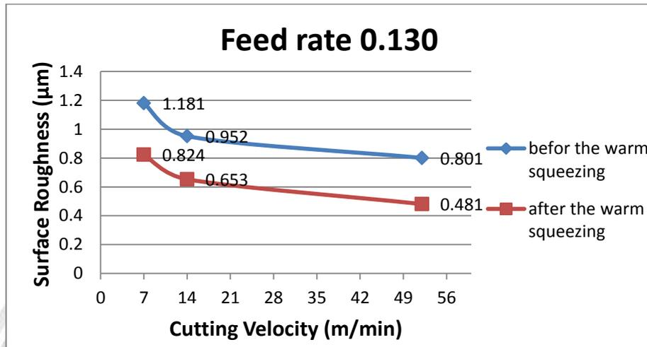
Figures (10): Effect of Cutting Speed on Sample Surface Roughness Before and After the Hot Press Used at a Cutting Depth  $d = 0.2$  mm and a Feed of (0.130 mm/rev)
