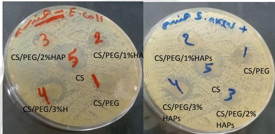
**Fig.6 Inhibition Zone Diameter of Neat CS, CS/PEG Blend, and Polymer Blend Nano Composites for E. coli and Staphylococcus Colony.**
