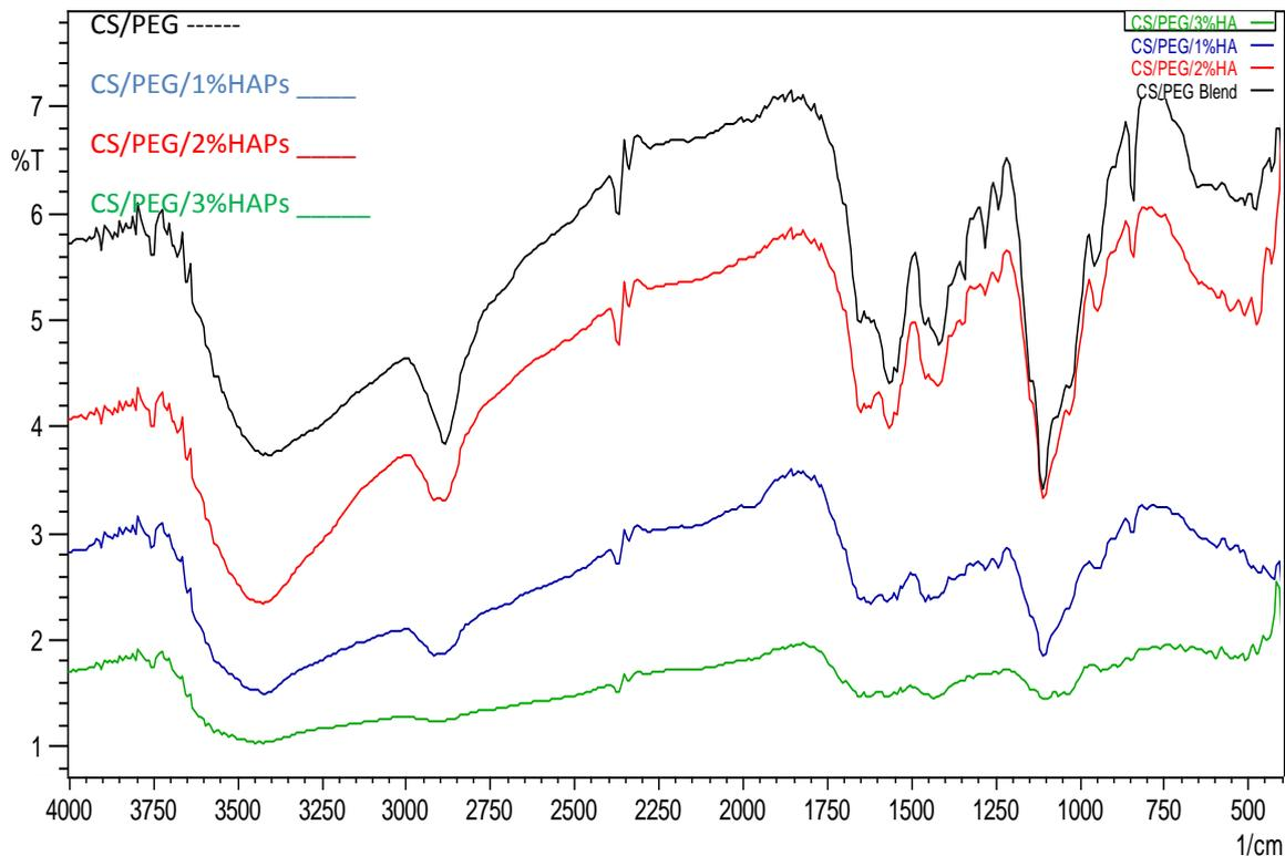
**Fig.1 FTIR Spectra (CS/PEG) and (CS/PEG) with HANPs% Nano Composite**
