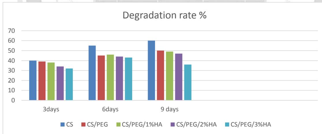
**Fig.5 Degradation Rate for CS, CS/PEG Blend, Nanocomposite with HANPs wt% and Hybrid Nanocomposite**
