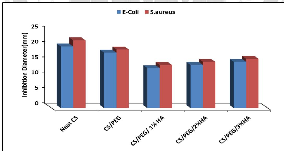
**Fig.7 Inhibition Diameter of Neat CS, CS/PEG Blend, and Nanocomposites as a Function of HANPs-Nanoparticles Content in Composite**
