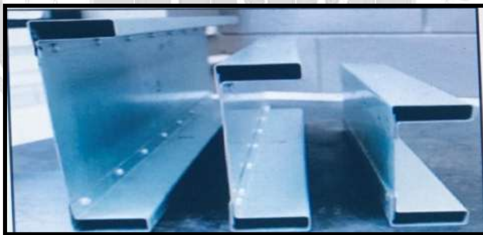
Figure (1): Rivet fastened rectangular hollow flange channel beam [4]
