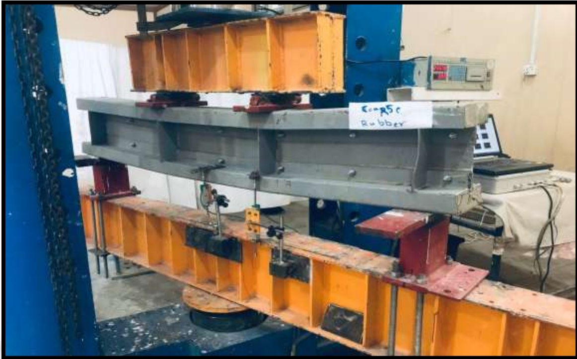
Figure (13): Failure of CFS I-beam strengthened the rectangular hollow flange by normal concrete has been replaced coarse aggregate with 30% coarse rubber(A60CR)
