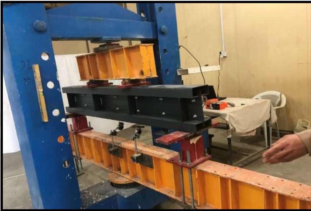
Figure (6): Testing CFS I-beam with rectangular hollow flange (A60)
