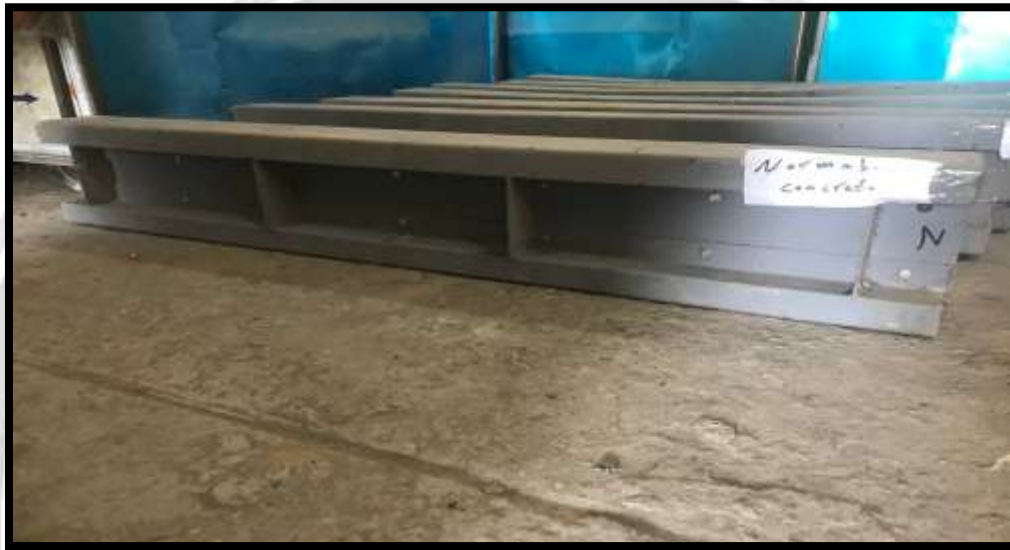
Figure (9): Failure of CFS I-beam strengthened the rectangular hollow flange by normal concrete(A60NC)
