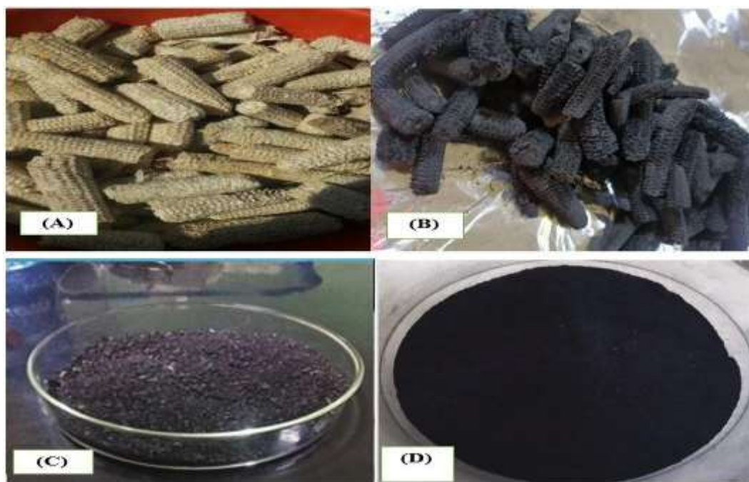
Figure 1: Macrostructural images of corn cob in different forms (a) dried-bulk corn cobs; (b) carbonized corn cob at 400 °C; (c) ground carbonized corn cobs; and (d) activated carbon from carbonized corn cob.
