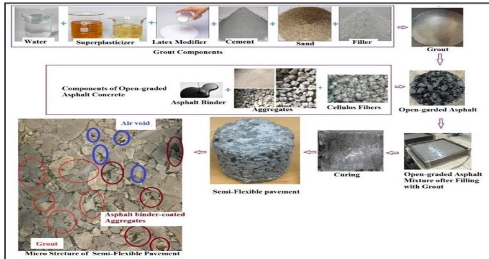
Figure 1. A Depiction Of The Blending Process For Semi-Flexible Pavements [10].
