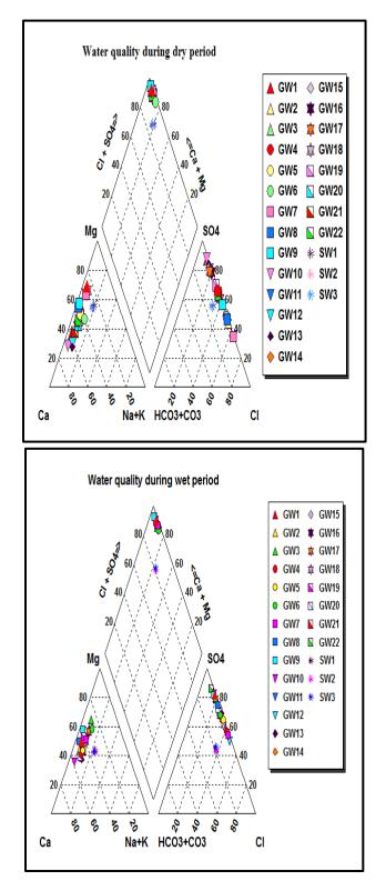
Figure (5): The water type of GW for two periods based on Piper diagram.
