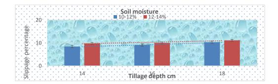
Fig 3. The effect of soil moisture and tillage depth on the slippage percentage %
