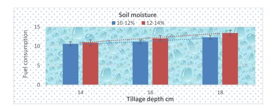
Fig 2. The effect of soil moisture and tillage depth on the fuel consumption L.ha<sup>-1</sup>
