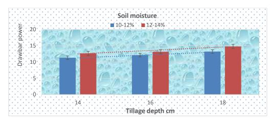
Fig 6. The effect of soil moisture and tillage depth on the drawbar power Kw .
