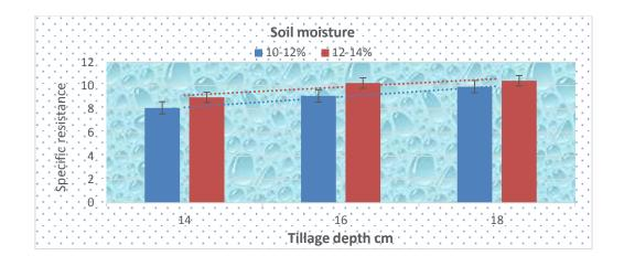
Fig 7. The effect of soil moisture and tillage depth on the specific resistance N.cm<sup>-2</sup>.
