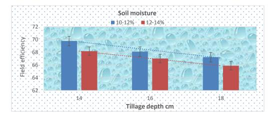
Fig 5. The effect of soil moisture and tillage depth on the field efficiency % .
