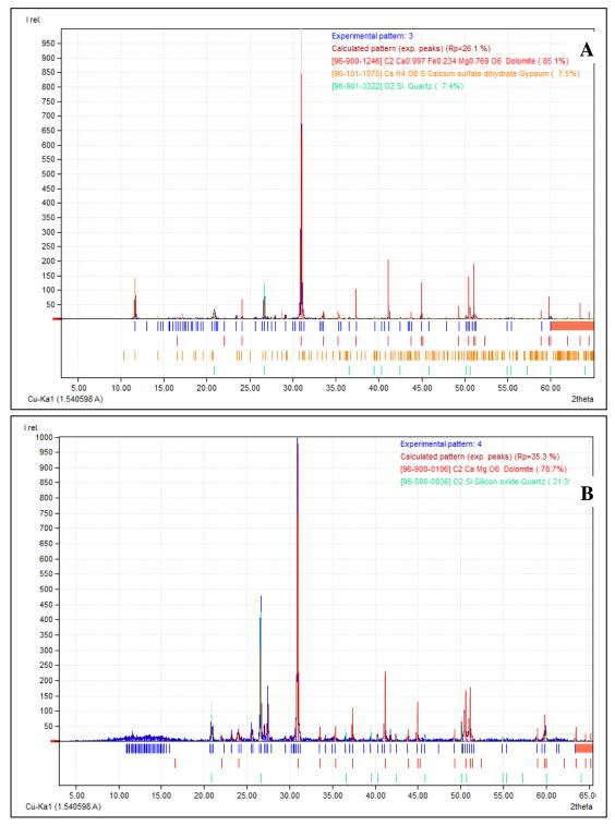
Figure 2: Diffractograms of carbonate units show mineralogical composition. A) Carbonate breccias. B) Stromatolite dolomite.
