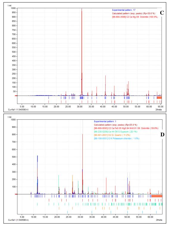
Figures 3: Diffractograms of carbonate units show mineralogical composition. C) Massive dolomite. D) Gypsiferous dolomite.
