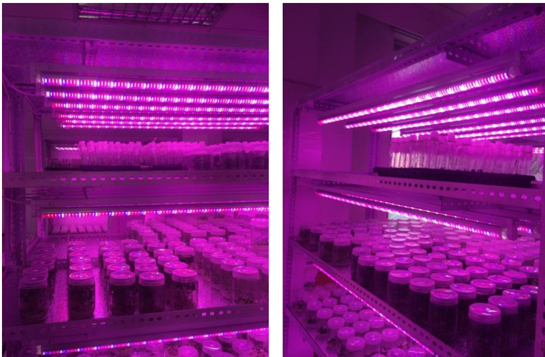
Fig 1. Growth of seedling under combinations of LED light (6:2:1), ((5:2:0), (4:1:1) and (3:1:1) with light intensity (500, 1000, 1500 and 2000 lux)
