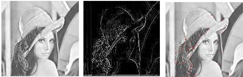
(B) Red Band image and its Edges computed using Laplacian Edge Detector
