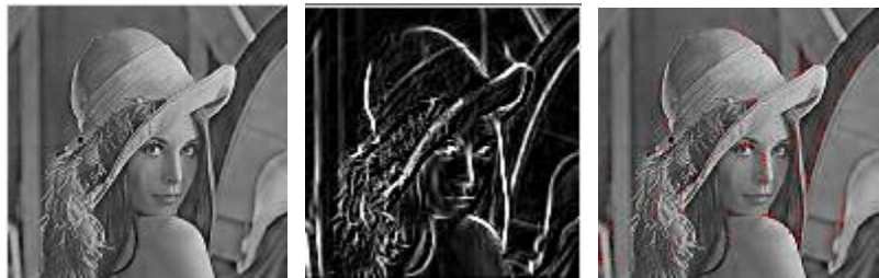
(D) Blue Band image and its Edges computed using Prewitt Edge Detector
